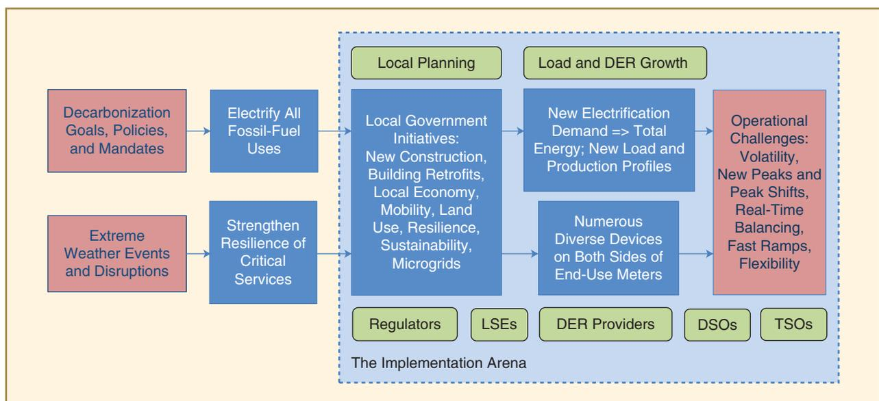
**figure 3.** The decarbonization and resilience goals drive new electrification demand and growth of DERs and could add to operational challenges and costly infrastructure needs unless shaped through incentives and grid services opportunities. LSEs: load-serving entities.
